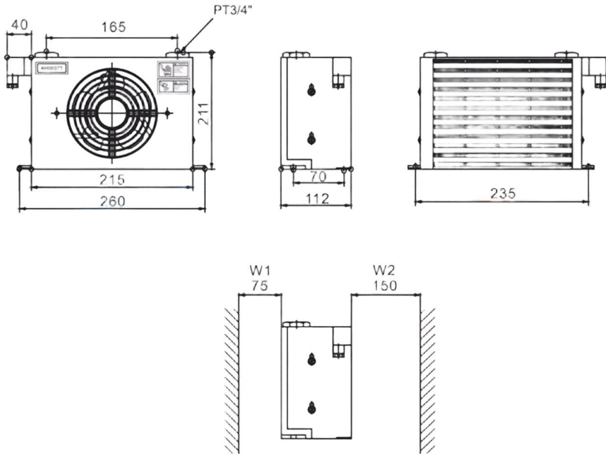
W1 is the min. distance between air inlet and obstacle
